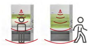
Intelligent monitoring of operation and automatic regulation of air supply
